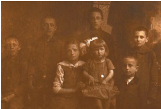
Photo 3. Gelatine-silver photograph with visible silver image degradation ( silver mirroring ), locally mechanically removed. Top: reproduction of the original print taken with a Canon EOS 5D Mark III digital camera. Below, the image obtained with MSI imaging (processing in HOKU software) (photo A. Seweryn)
